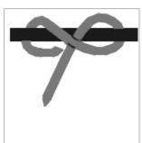
Then bring the running end forward over its own standing part. Pass the running end once more around the power cable and bring the running end in between the strap and the power cable.
