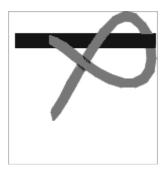
Pass the running end of the strap in front of the power cable and around it.
