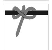
Tighten the Clove hitch by pulling on the running end.
