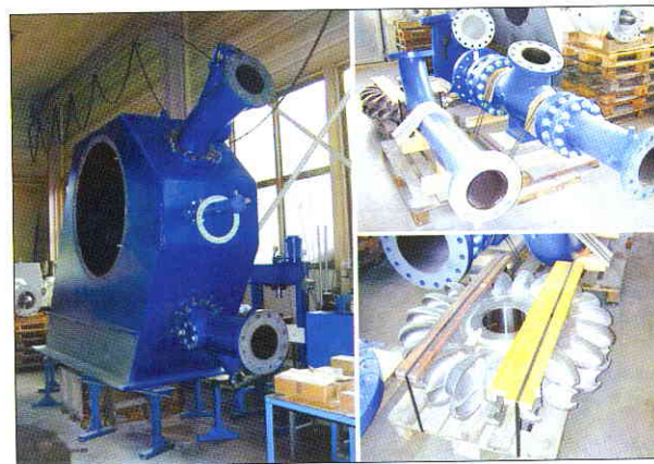
Fig. 2: Turbine components ready for shipment to Elandsrand mine. Output 3830 kW, head 620 m, speed 1500 rpm.
