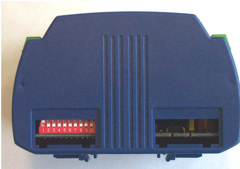
DIP switch for setting addresses (address 1 shown here)
